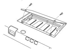
Figure 2-5 Accessing the Memory Slot
